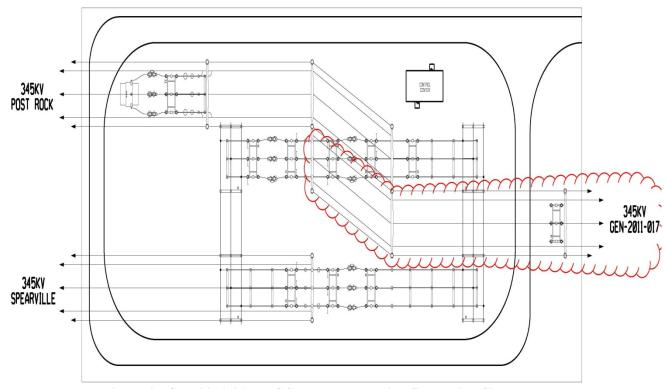
Figure 2 Gen-2011-017 ITCGP Interconnection Substation Site Plan
