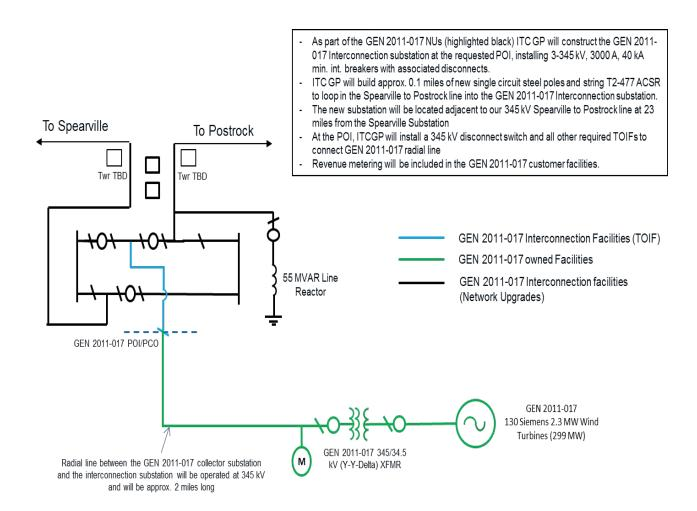
Figure 1 Gen-2011-017 ITCGP Interconnection Substation One Line
